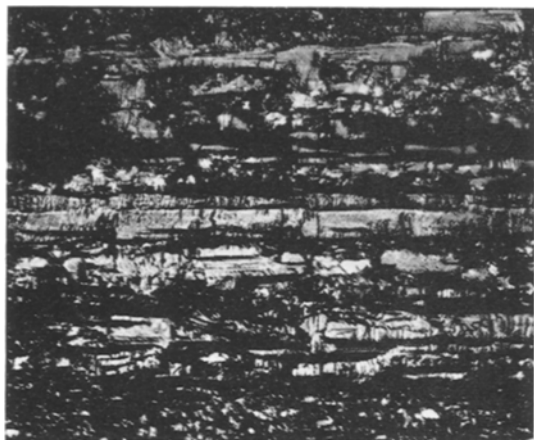
Figure 9 As-ground surface of a crystal ground wet with the diamond wheel at a medium rate of material removal ( d = 12.7 \mu\text{m} , V = 0.42 \text{ cm sec}^{-1} ) ( \times 160 ).
